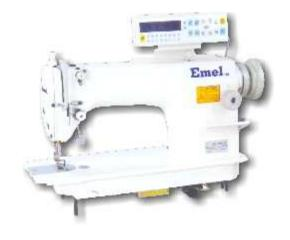
This model is equipped with automatic thread trimmer, automatic needle positioner, automatic thread wipe and many other sewing modes It is applied to sewing modes. It is applied to sewing shirt, uniforms and sportswears, and also applied to sewing port folios, purses, shoes, jeans and other medium-heavy weight materials, esp. Suitable for sewing trade marks, pockets, sleeve-cuffs, etc. It can be operated with high quality and high efficiency.
