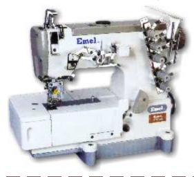
This machine is for regular cover stitching and can be equipped with various attachments for different sewing such as: tape binding.covering,thread plain seaming etc This machine is suitable for knitted underwear, sports, shirts and trousers,etc. This machine adopts complete-closed auto lubrication system, main drive adopts timings belt to assure high speed and lower noise.
