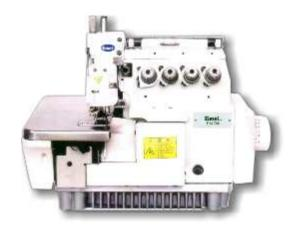
EM 700-04: 2-needle overedger for plain seaming attaching tape as well as plain seaming on light to medium fabrics. For sewing T-shirts,underwear,casual wear,sweat shirts and similar garments. Equipped with presser foot for attaching tape, the machine can perform tape attaching as well as plain seaming. Also equipped with an uncurler.
