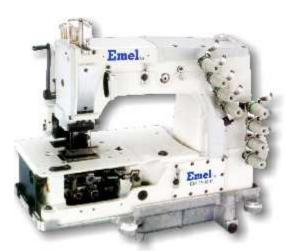
Flat Bed, 4 Needle, Double chain Stitch Machine for attaching waist bands.
