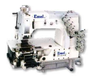
Flat Bed, 4 Needle Double Chain stitch machine for attaching. Elastic (with front feeding mechanism and rear puller).
